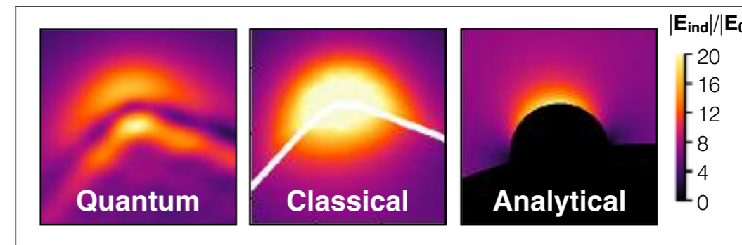
Zoom-in of the induced near-field around an atomic-scale feature, for atomistic quantum calculations based on linear-response time-dependent density functional theory (LR-TDDFT), calculations within a local classical description using the boundary element method (BEM), and a simplified classical model addressing the multiscale nature of the picocavities.
